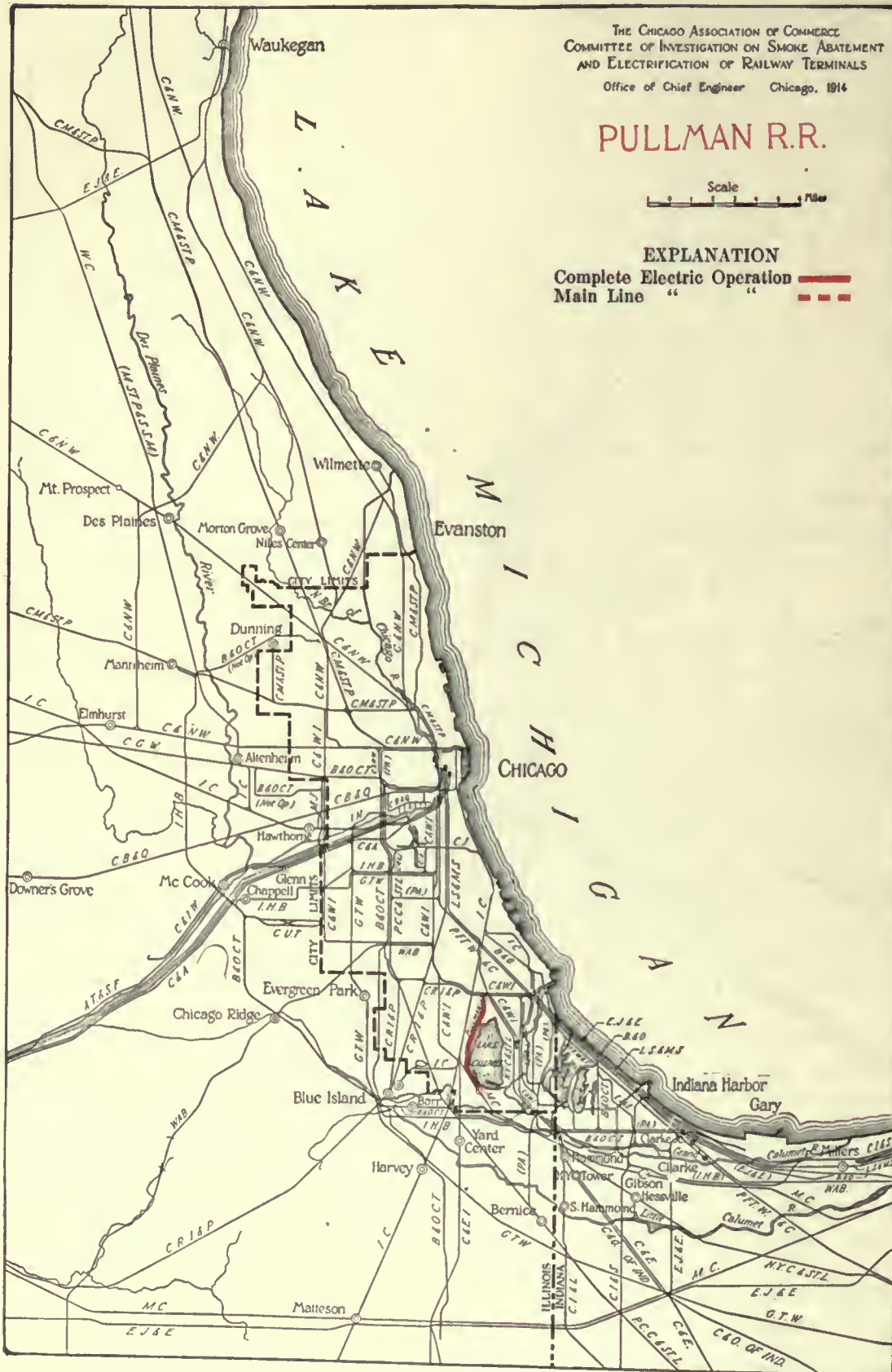
FIG. 573. TRACKAGE TO BE ELECTRIFIED BY THE PULLMAN RAILROAD
